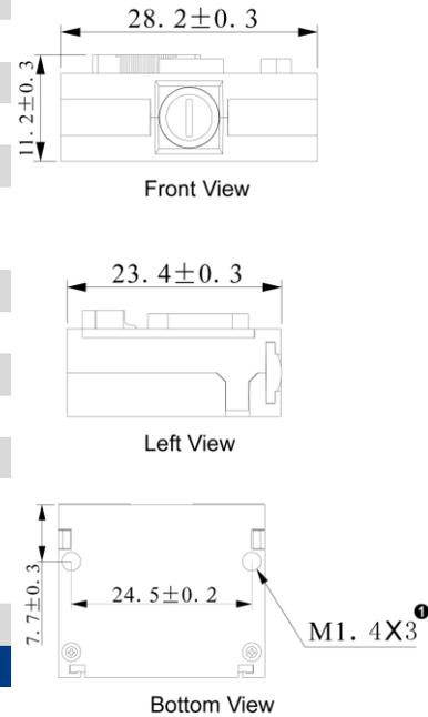
① Note: Machine Skew Diameter=1.4mm, Depth≤3mm
