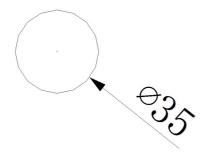
Requiring  $\phi 35$  hole, GB812 nut can be used to fix the column
