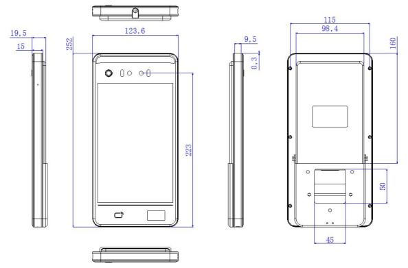
The deice package contains a wall mount bracket, plastic expansion screws, and tools. The following pic shows the size of the wall mount bracket
