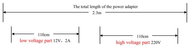
insufficient power supply at the host terminal of the device, causing abnormal phenomena such as repeated restarts and crashes. If the power source is far away from the device, you can extend the power cord (high voltage part).
